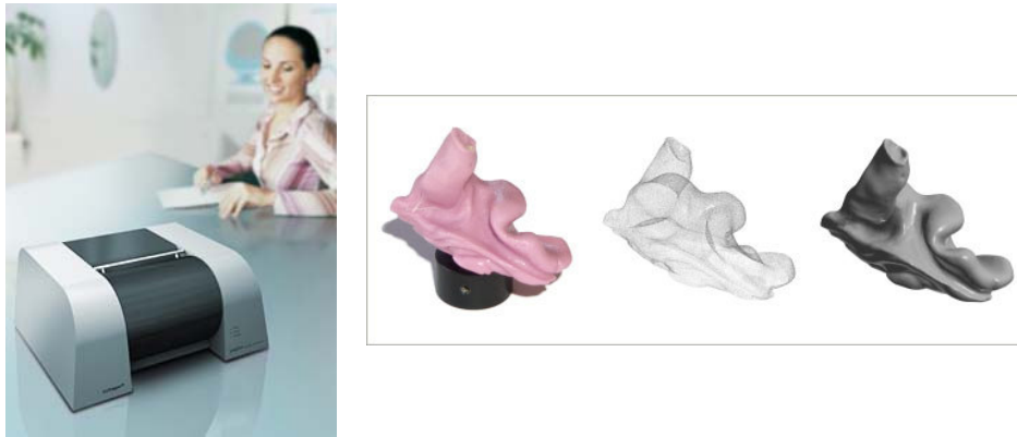
Figure 3.8: (left) Legato scanner from 3Shape. (right) An ear impression (physical object), the digital model shown as a wireframe and finally the shaded digital model.
