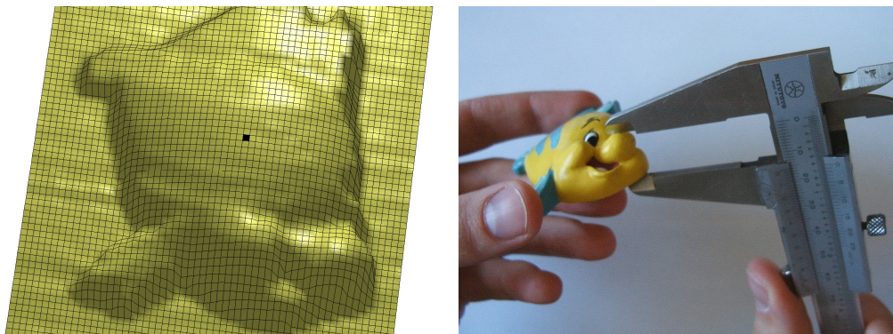
Figure 7.19: (left) The reconstructed fridge magnet fish with a single surface patch marked. The patch is moveable and average height of the patch is continually displayed. (right) Distinct points on the fish is measured using a slide gauge.
